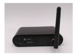
There is status lamp on transmitter, it have 7 colors, corresponding to 7 wireless dmx channels in light. .
